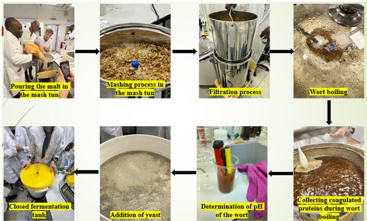
Figure 3. Flowchart of beer processing
